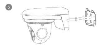
Pull wires through and make all necessary connections.
