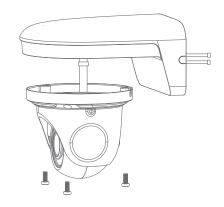
Separate the wall mount from the mounting template.
