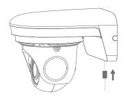
Connect the wall mount to the mounting bracket until secured. Use the small screw at the bottom of the wall mount to complete the installation.
